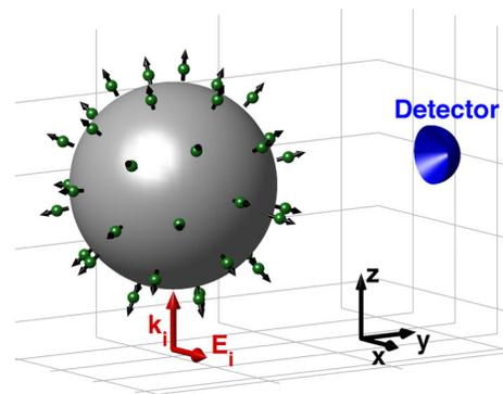
FIG. 1 (color online). Schematics of the system under study: a metal nanoparticle is surrounded by a collection of quantum emitters that are homogeneously distributed in a spherical shell and whose dipole orientations are radial.
